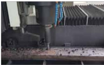
**Cutting condition**  $vc\text{ (m/min)}=60, fn\text{ (mm/rev)}=0.25, ap\text{ (mm)}=50$ , wet
