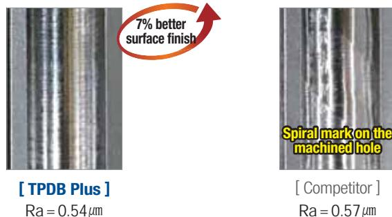
» Good surface finish due to stable chip shape and chip evacuation
