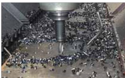
**Cutting condition**  $vc\text{ (m/min)}=70, fn\text{ (mm/rev)}=0.25, ap\text{ (mm)}=24$ , wet
