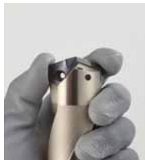
Lightly press the insert while screwing to prevent it from rotating.
