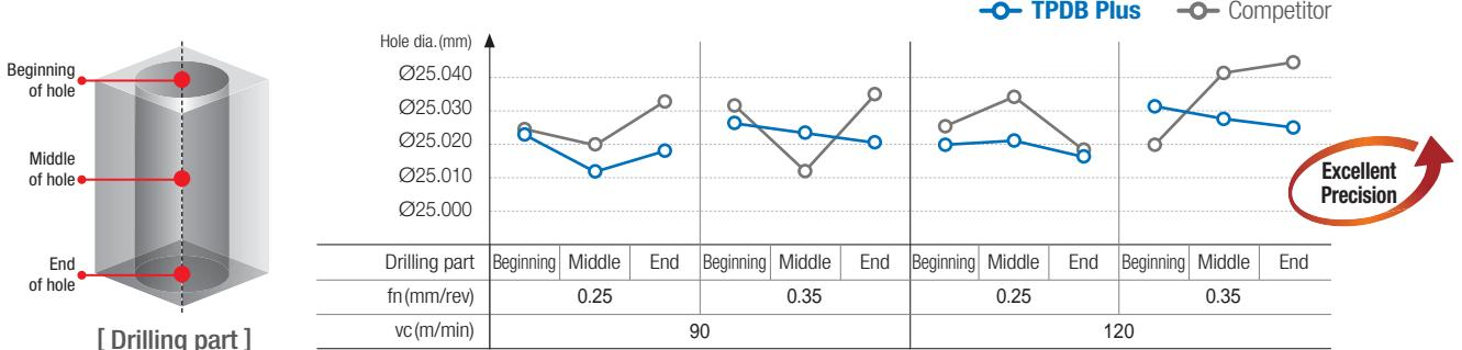
» High precision cutting due to stable chip evacuation
