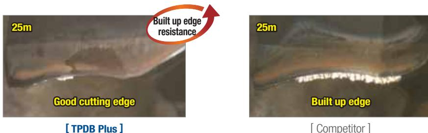
» Sharper cutting edge than competitor's improves built up edge resistance and tool life.
