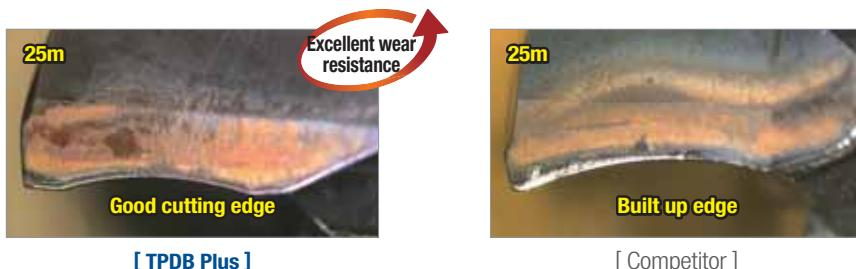
» Improved built up edge and chipping resistance lead stable wear on TPDB Plus insert's edge and obtain longer Max. tool life.
