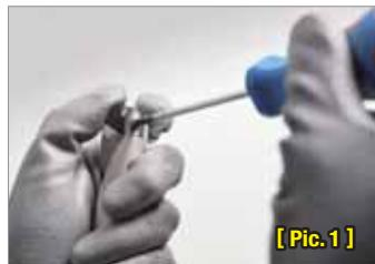
Put an insert on the tip seat of the holder.
