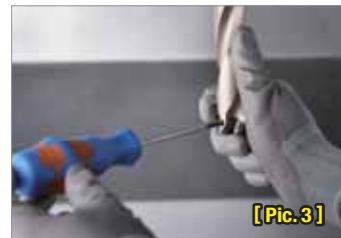
Put a new insert on the tip seat.
