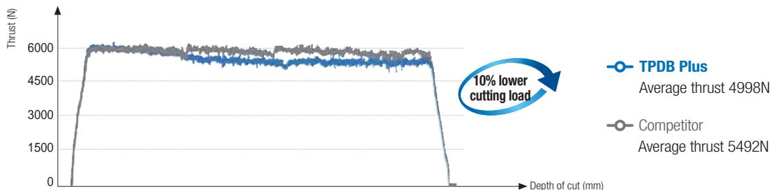
» Secured stable cutting load with excellent chip evacuation through applying low cutting resistance cutting edge and high helix flutes
