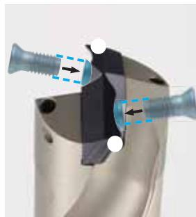
Screw the screws in the order of → to ←, which put screws first and tighten them in turn.
