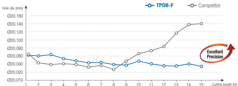
» Cutting edge with low cutting load enhances high precision.
