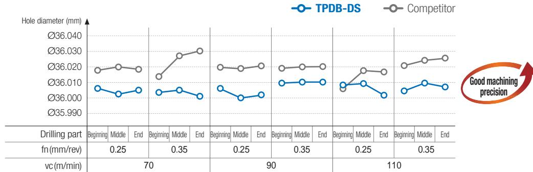
» Improved machining precision through double margin and stable chip evacuation
